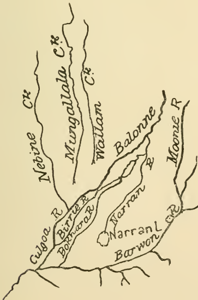
Diagram showing multiplicity of channels of an inland river in level country.
